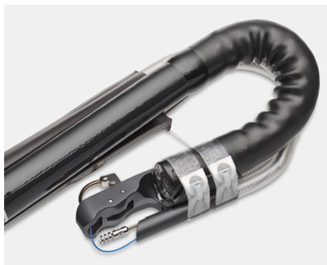
Figure 8. The Overstitch NXT OTSS system, demonstrating 210-degree retroflexion using MaxFlex. The incremental retroflexion is achieved using a pull-string mechanism attached to the control handle (not pictured). Courtesy of Boston Scientific.
